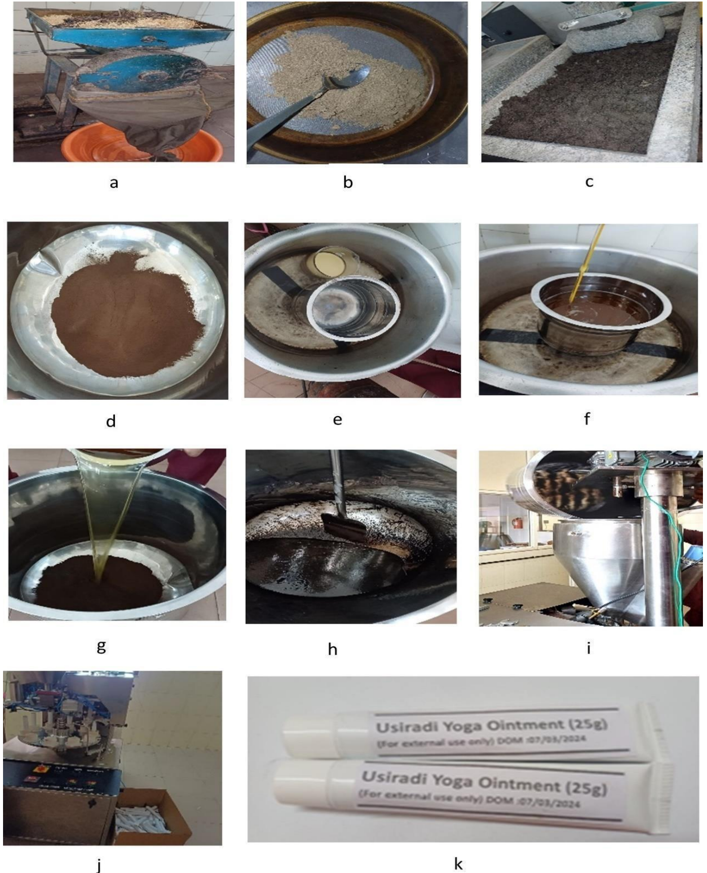
Figure 2: Stages of preparation of Usiradi Yoga Ointment a) Powdering of Ingredients b) Sieving through Sieve No.85 c) Bhavana in Gomutra arka d) Fine powder of Gomutra arka bhavita usiradi churna e) Melting of liquid paraffin and bees wax in water bath f) Reading ambient temperature of mixture of bees wax and liquid Paraffin g) Transferring the warm mixture into active ingredient ( Usiradi Powder ) h) Stirring of the mixture i) Transferring the mixture into ointment Tube filling machine j) Tube filling of ointment k) Usiradi Yoga Ointment .
