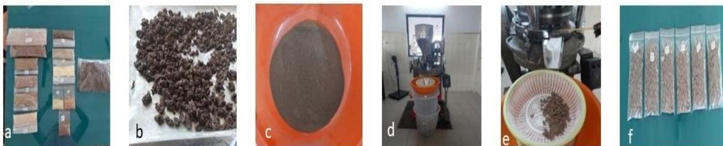
a. Fine powders of individual drugs, b. Fine powders with excipients, c. Granulated mixture, d. Tablet making machine, e. Dry compression of tablets, f. Six sets of tablets prepared
